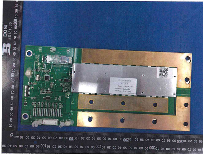
Picture 5. Protection board view
